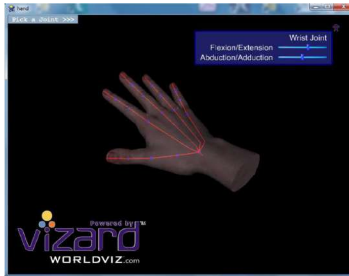
Figure 3.2: Screenshot of the 3D virtual visualization tool implemented to demonstrate the kinematic model of the human hand. The software tool is available online [Martins, 2009a] (url: http://www.rmartins.net/phd-docs/st01/ ).
