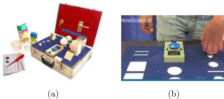
Figure 3.14: Southampton Hand Assessment Protocol (SHAP) [Adams et al., 2009]: a) complete kit. b) demonstration of assessment of hand function using the kit.
