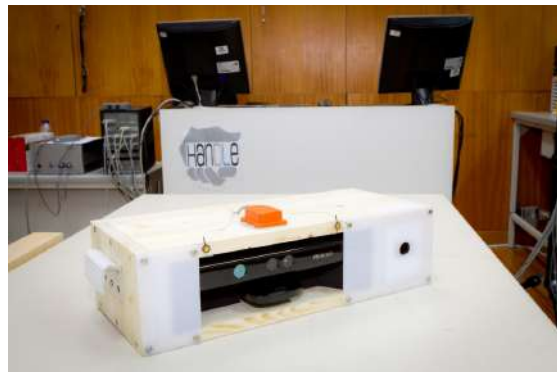
Figure 4.5: Microsoft Kinect integrated in a wood box.
