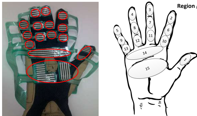
Figure 5.4: Representation of the fifteen spatial segments Region_i and their correspondence with the sensing elements of the instrumented glove.
